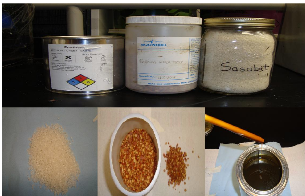
Figure 1: Additives (from left to right) a) Sasobit® b) Rediset™ c) Evotherm J1
